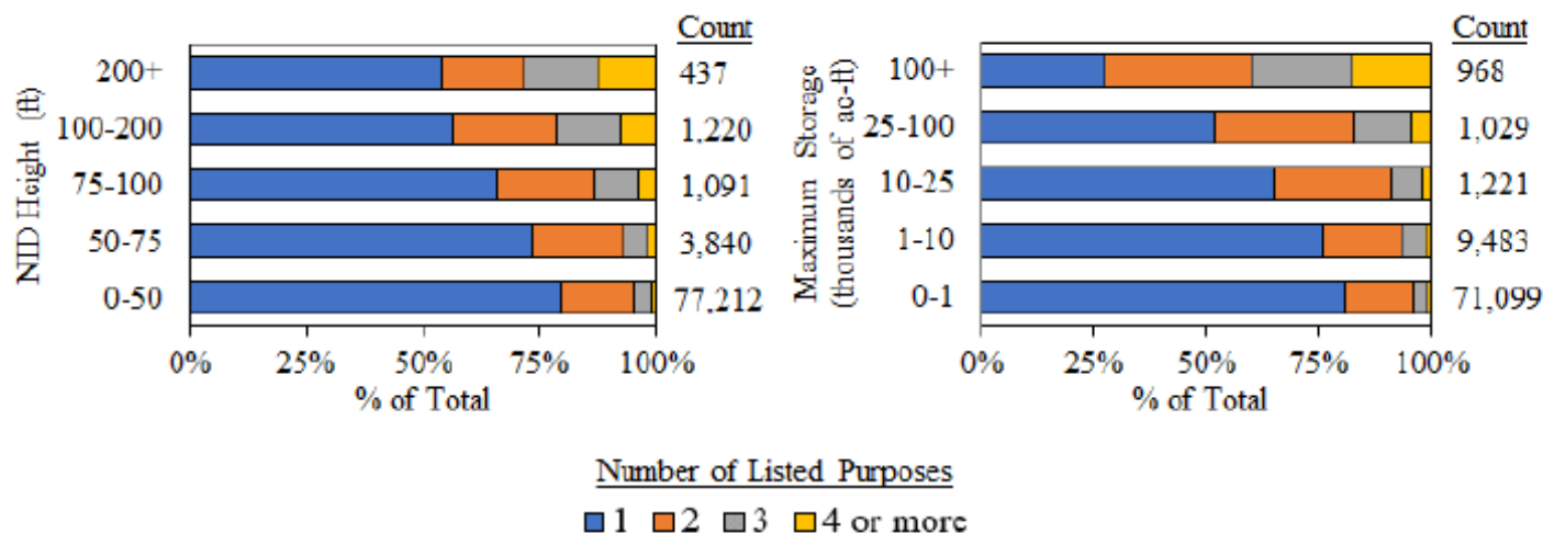
Figure 4. Number of listed purposes by NID height (left) and maximum storage (right) based on 2016 NID data. 7
